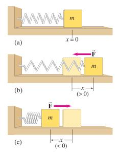
**FIGURE 11–1** An object of mass *m* oscillating at the end of a uniform spring. The force  $\vec{\mathbf{F}}$  on the object at the different positions is shown above the object.
