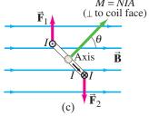
FIGURE 20-34 Calculating the torque on a current loop in a magnetic field  $\vec{\mathbf{B}}$ . (a) Loop face parallel to  $\vec{\mathbf{B}}$  field lines; (b) top view; (c) loop makes an angle to  $\vec{\mathbf{B}}$ , reducing the torque since the lever arm is reduced.
