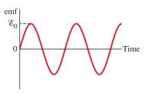
FIGURE 21-18 An ac generator produces an alternating current. The output emf  $\mathscr{E} = \mathscr{E}_0 \sin \omega t$ , where  $\mathcal{E}_0 = NA\omega B$  (Eq. 21–5).
