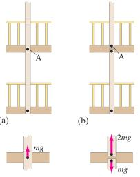
(d) Forces on pins (c) Force on pin A exerted by at A exerted by vertical rod vertical rods
