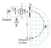
FIGURE 20-41 Bainbridge-type mass spectrometer. The magnetic fields B and B' point out of the paper (indicated by the dots).
