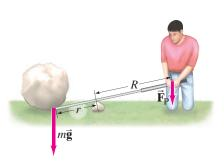
FIGURE 9-6 Example 9-3. A lever can "multiply" your force.
