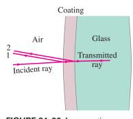
FIGURE 24–36 Lens coating, Example 24-12. Incident ray of light is partially reflected at the front surface of a lens coating (ray 1) and again partially reflected at the rear surface of the coating (ray 2), with most of the energy passing through as the transmitted ray into the glass.
