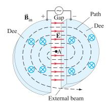
FIGURE 32-2 Diagram of a cyclotron. The magnetic field, applied by a large electromagnet, points into the page. The protons start at A, the ion source. The red electric field lines shown are for the alternating electric field in the gap at a certain moment.
