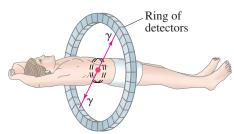
FIGURE 31-21 Positron emission tomography (PET) system showing a ring of detectors to detect the two annihilation  $\gamma$  rays  $(e^+ + e^- \rightarrow 2\gamma)$ emitted at 180° to each other.
