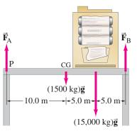
**FIGURE 9–8** A 1500-kg beam supports a 15,000-kg machine. Example 9–5.
