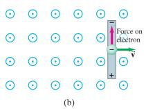
FIGURE 21–11 (a) A conducting rod is moved to the right on a U-shaped conductor in a uniform magnetic field  $\vec{B}$  that points out of the page. The induced current is clockwise. (b) Upward force on an electron in the metal rod (moving to the right) due to  $\vec{B}$  pointing out of the page; hence electrons can collect at the top of the rod, leaving + charge at the bottom.
