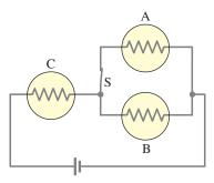
FIGURE 19-8 Example 19-6, three identical lightbulbs. Each yellow circle with -W- inside represents a lightbulb and its resistance.
