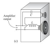
**FIGURE 21–42** (a) and (b): Two common uses for a capacitor as a filter. (c) Simple loudspeaker cross-over.
