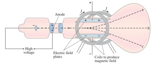
FIGURE 27–2 Cathode rays deflected by electric and magnetic fields. (See also Section 17-11 on the CRT.)
