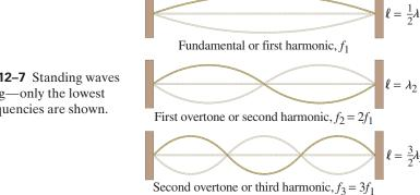
**FIGURE 12–7** Standing waves on a string—only the lowest three frequencies are shown.
