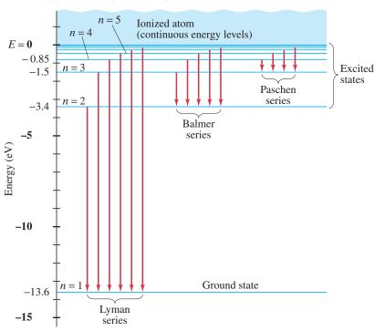
FIGURE 27–29 Energy-level diagram for the hydrogen atom, showing the transitions for the spectral lines of the Lyman, Balmer, and Paschen series (Fig. 27–25). Each vertical arrow represents an atomic transition that gives rise to the photons of one spectral line (a single wavelength or frequency).
