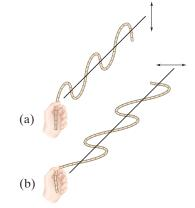
**FIGURE 24–38** Transverse waves on a rope polarized (a) in a vertical plane and (b) in a horizontal plane.
