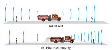
**FIGURE 12–19** (a) Both observers on the sidewalk hear the same frequency from the fire truck at rest. (b) Doppler effect: observer toward whom the fire truck moves hears a higher-frequency sound, and observer behind the fire truck hears a lower-frequency sound.
