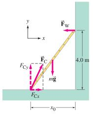
FIGURE 9-11 A ladder leaning against a wall. Example 9-7. The force  $\vec{\mathbf{F}}_C$  that the cement floor exerts on the ladder need not be along the ladder which (unlike a cord) is rigid.
