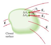
**FIGURE 16–44** Electric field lines passing through a closed surface. The surface is divided up into many tiny areas,  $\Delta A_1$ ,  $\Delta A_2$ , ..., and so on, of which only two are shown.
