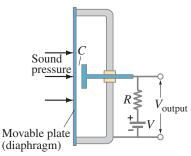
**FIGURE 17–16** Diagram of a condenser microphone.
