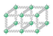
**FIGURE D-5** The atoms in a crystalline solid can vibrate about their equilibrium positions as if they were connected to their neighbors by springs. (The forces between atoms are actually electrical in nature.)
