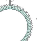
FIGURE 20-44 Iron-core toroid.
