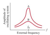
**FIGURE 11–18** Amplitude as a function of driving frequency *f*, showing resonance for lightly damped (A) and heavily damped (B) systems.
