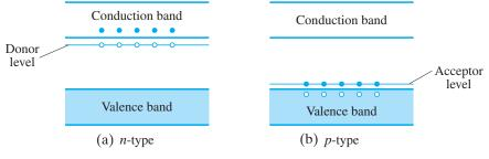
**FIGURE 29–28** Impurity energy levels in doped semiconductors.
