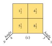
FIGURE 25-46 Reconstructing the image using projections in an iterative procedure.
