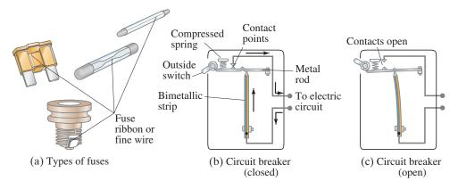
Household circuits are designed with the various devices connected so that each receives the standard voltage (Fig. 18–20) from the electric company (usually 120 V in the United States). Circuits with the devices arranged as in Fig. 18–20 are called parallel circuits, as we will discuss in the next Chapter. When a fuse blows or circuit breaker opens, it is important to check the total current being drawn on that circuit, which is the sum of the currents in each device.
