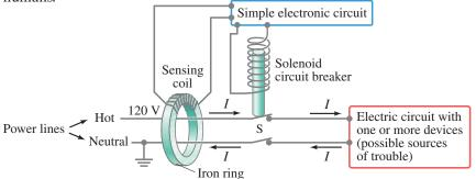
Electromagnetic induction is the physical basis of a GFCI. As shown in
