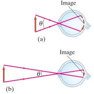
**FIGURE 25–16** When the same object is viewed at a shorter distance, the image on the retina is greater, so the object appears larger and more detail can be seen. The angle  $\theta$  that the object subtends in (a) is greater than in (b). *Note*: This is not a normal ray diagram because we are showing only one ray from each point.
