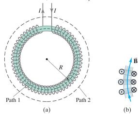
**FIGURE 20–60** Problem 49. (a) A toroid or torus. (b) A section of the toroid showing direction of the current for three loops: ⊙ means current toward you, and ⊗ means current away from you.
