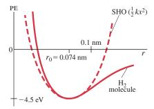
FIGURE 29-17 Potential energy for the H<sub>2</sub> molecule and for a simple harmonic oscillator (PE =  $\frac{1}{2}kx^2$ , with  $|x| = |r - r_0|$ .
