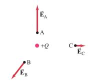
**FIGURE 16–30** Electric field vector, shown at three points, due to a single point charge Q. (Compare to Fig. 16–23.)
