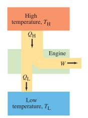
FIGURE 15–11 Schematic diagram of energy transfers for a heat engine.
