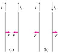
**EXAMPLE 20–12** Force between two current-carrying wires. The two wires of a 2.0-m-long appliance cord are 3.0 mm apart and carry a current of 8.0 A. Calculate the force one wire exerts on the other.
