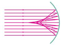
FIGURE 23-13 Parallel rays striking a concave spherical mirror do not intersect (or focus) at precisely a single point. (This "defect" is referred to as "spherical aberration.")
