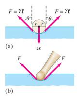
**FIGURE 10–36** Surface tension acting on (a) a sphere, and (b) an insect leg. Example 10–15.
