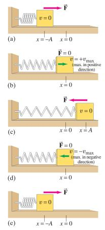
**FIGURE 11–2** An object oscillating on a frictionless surface, indicating the force on the object and its velocity at different positions of its oscillation cycle.
