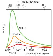
**FIGURE 27–4** Measured spectra of wavelengths and frequencies emitted by a blackbody at three different temperatures.
