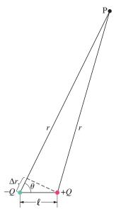
FIGURE 17-12 Electric dipole. Calculation of potential V at point P.
