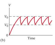
The intermittent windshield wipers of a car can also use an RC circuit. The RC time constant, which can be changed using a multi-positioned switch for different values of R with fixed C, determines the rate at which the wipers come on.
