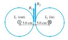
**EXAMPLE 20–10** Magnetic field midway between two currents. Two parallel straight wires 10.0 cm apart carry currents in opposite directions (Fig. 20–24). Current  $I_1 = 5.0$  A is out of the page, and  $I_2 = 7.0$  A is into the page. Determine the magnitude and direction of the magnetic field halfway between the two wires.
