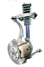
FIGURE 11-4 Photo of a car's spring. (Also visible is the shock absorber, in blue—see Section 11-5.)
