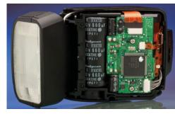
FIGURE 17-20 A camera flash unit. The  $660-\mu F$  capacitor is the black cylinder.
