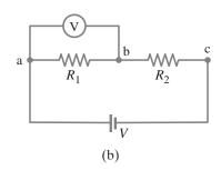
🖖 C A U T I O N Measurements affect the quantity being measured
