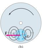
**FIGURE 21–20** Production of eddy currents in a rotating wheel. The gray lines in (b) indicate induced current.
