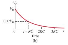
**EXAMPLE 19–13** A discharging RC circuit. If a charged capacitor,  $C = 35 \,\mu\text{F}$ , is connected to a resistance  $R = 120 \,\Omega$  as in Fig. 19–21a, how much time will elapse until the voltage falls to 10% of its original (maximum) value?
