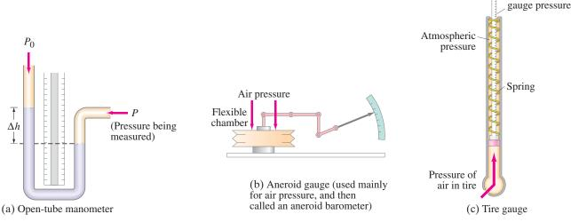
**FIGURE 10–7** Pressure gauges: (a) open-tube manometer, (b) aneroid gauge, and (c) common tire pressure gauge.
