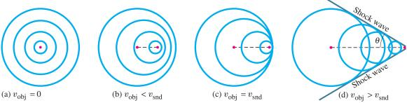
**FIGURE 12–23** Sound waves emitted by an object (a) at rest or (b, c, and d) moving. (b) If the object's velocity is less than the velocity of sound, the Doppler effect occurs. (c) At  $v_{\rm obj} = v_{\rm snd}$ , the waves pile up in front, forming a "sound barrier." (d) If the object's velocity is greater than the velocity of sound, a shock wave is produced.
