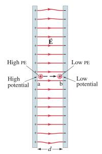
**FIGURE 17–1** Work is done by the electric field  $\vec{E}$  in moving the positive charge from position a to position b.
