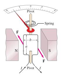
FIGURE 20-35 Galvanometer.
