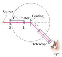
FIGURE 24-27 Spectrometer or spectroscope.
