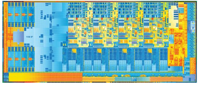
This computer processor chip contains over 1.4 billion transistors, plus diodes and other semiconductor electronic elements, all in a space of about 1 cm<sup>2</sup>. It uses 22-nm technology, meaning the "wires" (conducting lines) are 22 nm wide.
