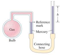
**FIGURE 13–8** Constant-volume gas thermometer.
