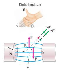
FIGURE 20-15 Force on charged particles due to a magnetic field is perpendicular to the magnetic field direction. If  $\vec{\mathbf{v}}$  is horizontal, then  $\mathbf{F}$  is vertical. The right-hand rule is shown for the force on a positive charge, +q.
