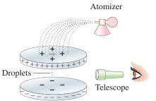
FIGURE 27–3 Millikan's oil-drop experiment.
