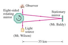
**FIGURE 22–10** Michelson's speed-of-light apparatus (not to scale).
