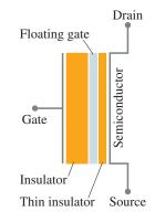
FIGURE 21–30 A floating gate nonvolatile memory cell (NVM).
