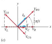
FIGURE 21-44 Phasor diagram for a series LRC circuit at (a) t = 0, (b) time tlater. (c) Projections on the x axis which give I,  $V_R$ ,  $V_C$ ,  $V_L$  at time t.
