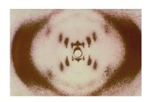
FIGURE 25–40 X-ray diffraction photo of DNA molecules taken by Rosalind Franklin in the early 1950s. The cross of spots suggested that DNA is a helix.
