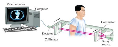
FIGURE 25-42 Tomographic imaging: the X-ray source and detector move together across the body, the transmitted intensity being measured at a large number of points. Then the "source-detector" assembly is rotated slightly (say, 1°) around a vertical axis, and another scan is made. This process is repeated for perhaps 180°. The computer reconstructs the image of the slice and it is presented on a TV or computer monitor.
