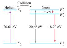
**FIGURE 28–20** Energy levels for He and Ne. He is excited in the electric discharge to the  $E_1$  state. This energy is transferred to the  $E'_3$  level of the Ne by collision.  $E'_3$  is metastable and decays to  $E'_2$  by stimulated emission.
