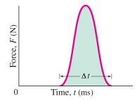
From Newton's second law, Eq. 7–2, the *net* force on an object is equal to the rate of change of its momentum:
