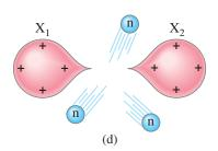
**FIGURE 31–3** Fission of a <sup>235</sup><sub>92</sub>U nucleus after capture of a neutron, according to the liquid-drop model.
