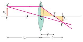
Let  $h_0$  and  $h_i$  refer to the heights of the object and image. Consider the two rays shown in Fig. 23–40 for a converging lens, assumed to be very thin. The right triangles FI'I and FBA (highlighted in yellow) are similar because angle AFB equals angle IFI'; so
