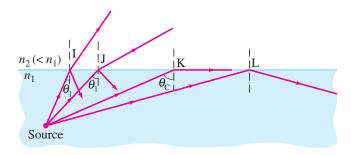
**FIGURE 23–26** Since  $n_2 < n_1$ , light rays are totally internally reflected if the incident angle  $\theta_1 > \theta_C$ , as for ray L. If  $\theta_1 < \theta_C$ , as for rays I and J, only a part of the light is reflected, and the rest is refracted.
