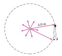
**FIGURE 31–16** Radiation spreads out in all directions. A person 4.0 m away intercepts only a fraction: her cross-sectional area divided by the area of a sphere of radius 4.0 m. Example 31-12.
