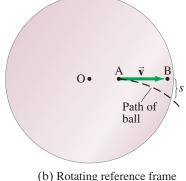
**FIGURE C–2** The origin of the Coriolis effect. Looking down on a rotating platform, (a) as seen from a nonrotating inertial reference frame, and (b) as seen from the rotating platform as frame of reference.
