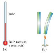
**FIGURE 13–5** (a) Mercury- or alcohol-in-glass thermometer; (b) bimetallic strip.
