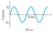
FIGURE 18-21 (a) Direct current, and (b) alternating current, as functions of time.
