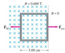
**FIGURE 21–9** Example 21–4. The square coil in a magnetic field  $B = 0.600 \,\mathrm{T}$  is pulled abruptly to the right to a region where B = 0. (The forces shown are discussed in the alternate solution at the end of Example 21–4.)
