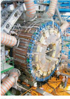
FIGURE 32-6 ATLAS, one of the large complex detectors at the LHC, is shown here as it was being built. In 2012 it was used to provide evidence for the Higgs boson. Note the people near the bottom. From the outside, the CMS detector at the LHC looks similar.
