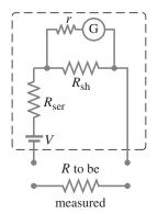
FIGURE 19–35 An ohmmeter.
