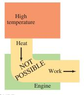
FIGURE 15-15 Diagram of an impossible perfect heat engine in which all heat input is used to do work.
