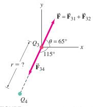
**FIGURE 16–21** Example 16–5 and Exercise D:  $Q_4$  exerts force  $(\vec{\mathbf{F}}_{34})$  that makes the net force on  $Q_3$  zero.
