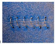
**FIGURE 20–28** (a) Magnetic field of a solenoid. The north pole of this solenoid, thought of as a magnet, is on the right, and the south pole is on the left. (b) Photo of iron filings aligning along  $\vec{\mathbf{B}}$  field lines of a solenoid with loosely spaced loops. The field is smoother if the loops are closely spaced.
