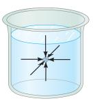
FIGURE 10-1 Pressure is the same in every direction in a nonmoving fluid at a given depth. If this weren't true, the fluid would be in motion.
