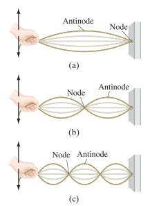
**FIGURE 11–40** Standing waves corresponding to three resonant frequencies.
