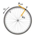
FIGURE 8-6 On a rotating wheel whose angular speed is increasing, a point P has both tangential and radial (centripetal) components of linear acceleration. (See also Chapter 5.)
