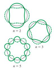
**FIGURE 27–31** (Repeated.) Standing circular waves for two, three, and five wavelengths on the circumference; *n*, the number of wavelengths, is also the quantum number.
