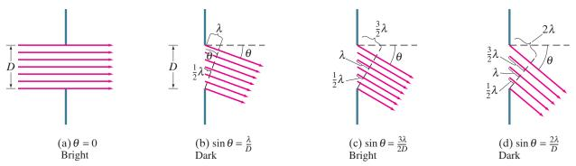
**FIGURE 24–20** Analysis of diffraction pattern formed by light passing through a narrow slit of width D.
