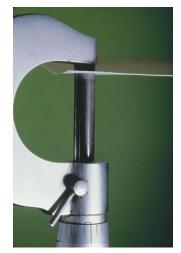
**FIGURE 1–11** Example 1–7. Micrometer used for measuring small thicknesses.
