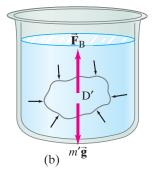
FIGURE 10–11 Archimedes' principle.
