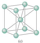
**FIGURE 29–19** Arrangement of atoms in (a) a simple cubic crystal, (b) face-centered cubic crystal (note the atom at the center of each face), and (c) body-centered cubic crystal. Each of these "cells" is repeated in three dimensions to the edges of the macroscopic crystal.
