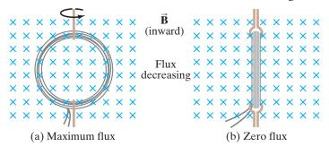
FIGURE 21-6 A current can be induced by rotating a coil in a magnetic field. The flux through the coil changes from (a) to (b) because  $\theta$  (in Eq. 21–1,  $\Phi = BA \cos \theta$ ) went from  $0^{\circ}$  (cos  $\theta = 1$ ) to  $90^{\circ}$  (cos  $\theta = 0$ ).
