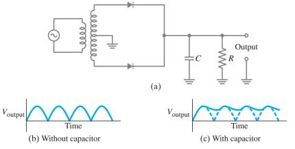
FIGURE 29–32 (a) Full-wave rectifier circuit (including a transformer so the magnitude of the voltage can be changed). (b) Output voltage in the absence of capacitor *C*. (c) Output voltage with the capacitor in the circuit.
