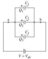
FIGURE 19-17 Capacitors in parallel:  $C_{eq} = C_1 + C_2 + C_3$ .
