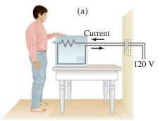
**FIGURE 19–26** (a) An electric oven operating normally with a 2-prong plug. (b) A short to a metal case which is ungrounded, causing a shock. (c) A short to the case which is grounded by a 3-prong plug; almost no current goes through the person.
