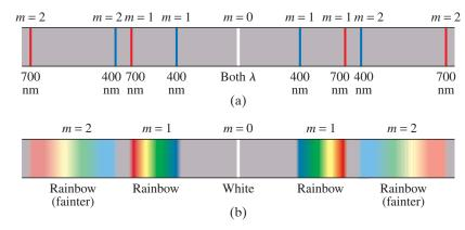
**FIGURE 24–26** Spectra produced by a grating: (a) two wavelengths, 400 nm and 700 nm; (b) white light. The second order will normally be dimmer than the first order. (Higher orders are not shown.) If the grating spacing is small enough, the second and higher orders will be missing.
