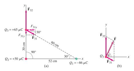
**EXAMPLE 16–4** Electric force using vector components. Calculate the net electrostatic force on charge  $Q_3$  shown in Fig. 16–20a due to the charges  $Q_1$  and  $Q_2$ .
