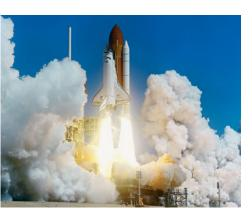
FIGURE 4-10 Another example of Newton's third law: the launch of a rocket. The rocket engine pushes the gases downward, and the gases exert an equal and opposite force upward on the rocket, accelerating it upward. (A rocket does not accelerate as a result of its expelled gases pushing against the ground.)
