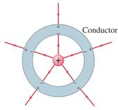
FIGURE 16-34 A charge inside a neutral spherical metal shell induces charge on its surfaces. The electric field exists even beyond the shell, but not within the conductor itself.
