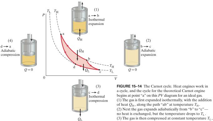
FIGURE 15–14 The Carnot cycle. Heat engines work in a cycle, and the cycle for the theoretical Carnot engine begins at point "a" on this PV diagram for an ideal gas. (1) The gas is first expanded isothermally, with the addition of heat  $Q_{\rm H}$ , along the path "ab" at temperature  $T_{\rm H}$ . (2) Next the gas expands adiabatically from "b" to "c" no heat is exchanged, but the temperature drops to  $T_L$ .
