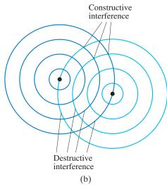
**FIGURE 11–38** (a) Interference of water waves. (b) Constructive interference occurs where one wave's maximum (a crest) meets the other's maximum. Destructive interference ("flat water") occurs where one wave's maximum (a crest) meets the other's miminum (a trough).
