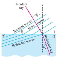
FIGURE 11-42 Refraction of waves passing a boundary.
