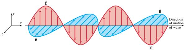
If the source voltage varies sinusoidally, then the electric and magnetic field strengths in the radiation field will also vary sinusoidally. The sinusoidal character of the waves is shown in Fig. 22-7, which displays the field directions and magnitudes plotted as a function of position along the direction of wave travel. Notice that  $\vec{\bf B}$  and  $\vec{\bf E}$  are perpendicular to each other and to the direction of wave travel.
