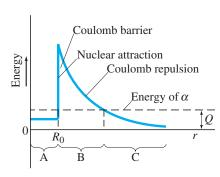
**FIGURE 30–12** Potential energy for alpha particle and nucleus, showing the "Coulomb barrier" through which the  $\alpha$  particle must tunnel to escape. The Q-value of the reaction is also indicated.
