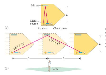
**FIGURE 26–6** Time dilation can be shown by a thought experiment: the time it takes for light to travel across a spaceship and back is longer for the observer on Earth (b) than for the observer on the spaceship (a).
