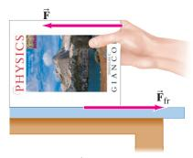
**FIGURE 4–3**  $\vec{\mathbf{F}}$  represents the force applied by the person and  $\vec{\mathbf{F}}_{fr}$  represents the force of friction.
