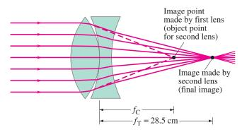
**FIGURE 23–45** Determining the focal length of a diverging lens. Example 23–16.
