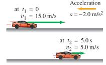
FIGURE 2-11 Example 2-6, showing the position of the car at times  $t_1$  and  $t_2$ , as well as the car's velocity represented by the green arrows. The acceleration vector (orange) points to the left because the car slows down as it moves to the right.
