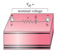
FIGURE 19-1 Diagram for an electric cell or battery.
