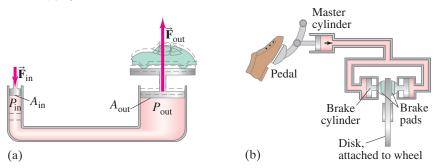
Figure 10–6b illustrates the brake system of a car. When the driver presses the brake pedal, the pressure in the master cylinder increases. This pressure increase occurs throughout the brake fluid, thus pushing the brake pads against the disk attached to the car's wheel.
