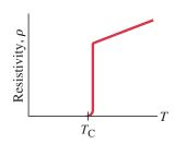
**FIGURE 18–26** A superconducting material has zero resistivity when its temperature is below  $T_{\rm C}$ , its "critical temperature." At temperatures above  $T_{\rm C}$ , the resistivity jumps to a "normal" nonzero value and increases with temperature as most materials do (Eq. 18–4).
