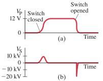
**FIGURE 21–24** A dc voltage turned on and off as shown in (a) produces voltage pulses in the secondary (b). Voltage scales in (a) and (b) are not the same.
