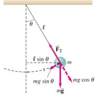
**FIGURE 11–12** Simple pendulum, and a free-body diagram.
