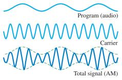
**FIGURE 22–14** In amplitude modulation (AM), the amplitude of the carrier signal is made to vary in proportion to the audio signal's amplitude.
