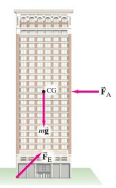
FIGURE 9-80 Forces on a building subjected to wind  $(\vec{\mathbf{F}}_{A})$ , gravity  $(m\vec{\mathbf{g}})$ , and the force  $\vec{\mathbf{F}}_{E}$ on the building due to the Earth if the building were just about to tip. Problem 61.
