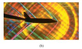
FIGURE 12-25 (a) The (double) sonic boom has already been heard by person A on the left. The front shock wave is just being heard by person B in the center. And both will shortly be heard by person C on the right. (b) Special photo of supersonic aircraft showing shock waves produced in the air. (Several closely spaced shock waves are produced by different parts of the aircraft.)
