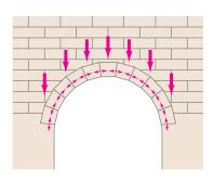
FIGURE 9-29 Stones in a round arch (see Fig. 9-28a) are mainly under compression.
