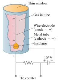
FIGURE 30-13 Diagram of a Geiger counter.
