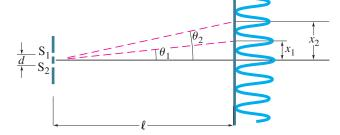
**CONCEPTUAL EXAMPLE 24–2** Changing the wavelength. (a) What happens to the interference pattern shown in Fig. 24–10, Example 24–1, if the incident light (500 nm) is replaced by light of wavelength 700 nm? (b) What happens instead if the wavelength stays at 500 nm but the slits are moved farther apart?
