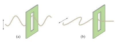
**FIGURE 24–39** (a) A vertically polarized wave passes through a vertical slit, but (b) a horizontally polarized wave will not.
