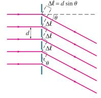
FIGURE 24-24 Diffraction grating.
