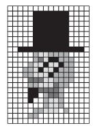
FIGURE 24-49 Example of an image made up of many small squares or pixels (picture elements).
