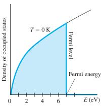
**FIGURE 29–21** At T = 0 K, all states up to energy  $E_{\rm F}$ , called the Fermi energy, are filled. (Shown here for copper.)
