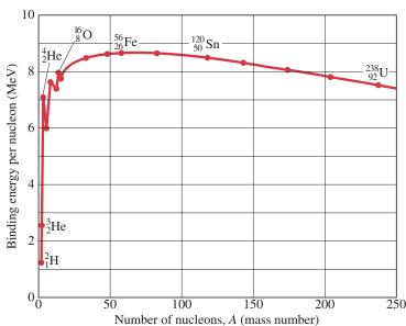
FIGURE 30–1 Binding energy per nucleon for the more stable nuclides as a function of mass number A.
