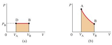
**FIGURE 15–7** Work done by a gas is equal to the area under the *PV* curve.
