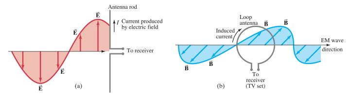
**FIGURE 22–18** Antennas. (a) Electric field of EM wave produces a current in an antenna consisting of straight wire or rods. (b) The moving and changing magnetic field induces an emf and current in a loop antenna.
