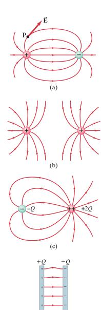
FIGURE 16-32 Electric field lines for four arrangements of charges.
