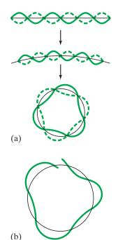
FIGURE 27-30 (a) An ordinary standing wave compared to a circular standing wave. (b) When a wave does not close (and hence interferes destructively with itself), it rapidly dies out.
