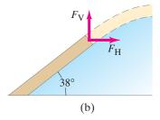
**FIGURE 9–34** Example 9–13. (a) The dome of the Small Sports Palace in Rome, built by Pier Luigi Nervi for the 1960 Olympics. (b) The force components each buttress exerts on the dome.
