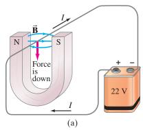
FIGURE 20-11 (a) Force on a current-carrying wire placed in a magnetic field  $\vec{\mathbf{B}}$ ; (b) same, but current reversed; (c) right-hand rule for setup in (b), with current  $\vec{I}$ shown as if a vector with direction.
