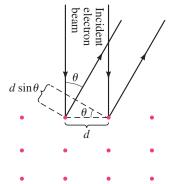
**FIGURE 27–13** Example 27–12. The red dots represent atoms in an orderly array in a solid.
