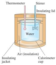
FIGURE 14-4 Simple water calorimeter.
