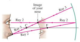
**FIGURE 23–18** You can see a clear inverted image of your face in a concave mirror when you are beyond C  $(d_0 > 2f)$ , because the rays that arrive at your eye are *diverging*. Standard rays 2 and 3 are shown leaving point O on your nose. Ray 2 (and other nearby rays) enters your eye. Notice that rays are diverging as they move to the left of image point I.
