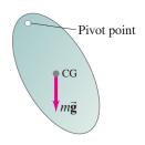
**FIGURE 7–24** The force of gravity, considered to act at the CG, causes this object to rotate about the pivot point; if the CG were on a vertical line directly below the pivot, the object would remain at rest.
