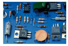
**FIGURE 18–11** Photo of resistors (striped), plus other devices on a circuit board.
