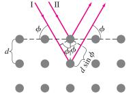
FIGURE 25-39 X-rays can be diffracted from many possible planes within a crystal.
