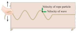
FIGURE 11–22 Wave traveling on a rope or cord. The wave travels to the right along the rope. Particles of the rope oscillate back and forth on the tabletop.
