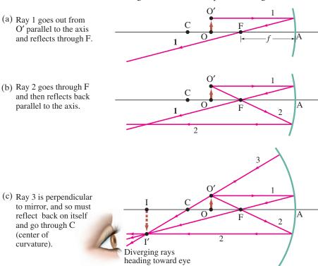
FIGURE 23-15 Rays leave point O' on the object (an arrow). Shown are the three most useful rays for determining where the image I' is formed. [Note that our mirror is not small compared to f, so our diagram will not give the precise position of the image.]
