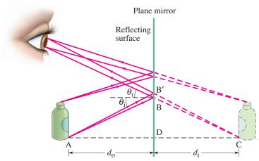
FIGURE 23-7 Formation of a virtual image by a plane mirror. Only the bundle of rays from the top and bottom of the object which reach the eye is shown.
