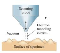
FIGURE 27–17 The probe tip of a scanning tunneling electron microscope, as it is moved horizontally, automatically moves up and down to maintain a constant tunneling current, and this motion is translated into an image of the surface.
