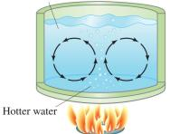
**FIGURE 14–8** Convection currents in a pot of water being heated on a stove.
