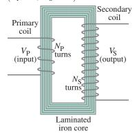
If the secondary coil contains more loops than the primary coil  $(N_{\rm S}>N_{\rm P})$ , we have a **step-up transformer**. The secondary voltage is greater than the primary voltage. For example, if the secondary coil has twice as many turns as the primary coil, then the secondary voltage will be twice that of the primary voltage. If  $N_{\rm S}$  is less than  $N_{\rm P}$ , we have a **step-down transformer**.
