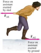
**FIGURE 4–13** Example 4–5. The horizontal forces on the assistant.
