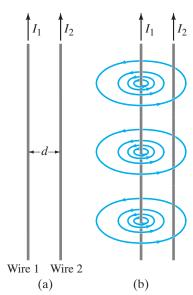
FIGURE 20-26 (a) Two parallel conductors carrying currents  $I_1$  and  $I_2$ . (b) Magnetic field  $\vec{\mathbf{B}}_1$  produced by  $I_1$ . (Field produced by  $I_2$  is not shown.)  $\vec{\mathbf{B}}_1$  points into page at position of  $I_2$ .
