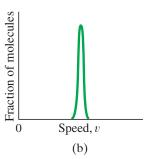
**FIGURE 15–19** (a) Most probable distribution of molecular speeds in a gas (Maxwellian, or random). (b) Orderly, but highly unlikely, distribution of speeds in which all molecules have nearly the same speed.
