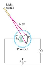
FIGURE 27-6 The photoelectric effect.
