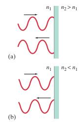
FIGURE 24-32 (a) Reflected ray changes phase by  $180^{\circ}$  or  $\frac{1}{2}$  cycle if  $n_2 > n_1$ , but (b) does not if  $n_2 < n_1$ .
