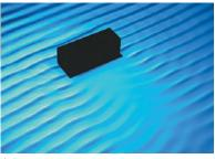
(b) FIGURE 11-45 Wave diffraction. In (a) the waves pass through a slit and into the "shadow region" behind. In (b) the waves are coming from the upper left. As they pass an obstacle, they bend around it into the
