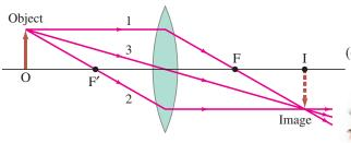
(c) Ray 3 passes straight through the center of the lens (assumed very thin). FIGURE 23-37 Finding the image by ray tracing for a converging lens. Rays are shown leaving one point on the object (an arrow). Shown are the three most useful rays, leaving the tip of the object, for determining where the image of that point is formed. (Note that the focal points F and F' on either side of the lens are the same distance f from the center of the lens.)
