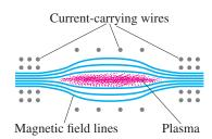
FIGURE 31-13 "Magnetic bottle" used to confine a plasma.
