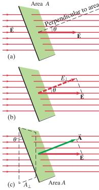
FIGURE 16-43 (a) A uniform electric field  $\vec{E}$  passing through a flat square area A. (b)  $E_{\perp} = E \cos \theta$  is the component of  $\vec{\mathbf{E}}$  perpendicular to the plane of area A. (c)  $A_{\perp} = A \cos \theta$  is the projection (dashed) of the area A perpendicular to the field  $\vec{\mathbf{E}}$ .
