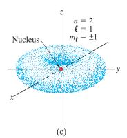
**FIGURE 28–9** Electron cloud, or probability distribution, for n = 2 states in hydrogen. [The donutshaped orbit in (c) is the sum of two dumbbell-shaped orbits, as in (b), along the x and y axes added together.]
