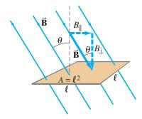
FIGURE 21–3 Determining the flux through a flat loop of wire. This loop is square, of side  $\ell$  and area  $A = \ell^2$ .
