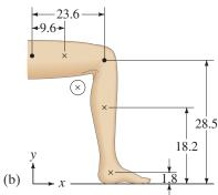
**FIGURE 7–26** Example 7–13: finding the CM of a leg in two different positions using percentages from Table 7–1. ( $\otimes$  represents the calculated CM.)
