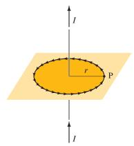
FIGURE 20-31 Circular path of radius *r*.
