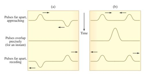
FIGURE 11-37 Two wave pulses pass each other. Where they overlap, interference occurs: (a) destructive, and (b) constructive. Read (a) and (b) downward (increasing time).
