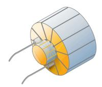
**FIGURE 20–39** Motor with many windings.
