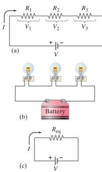
**FIGURE 19–3** (a) Resistances connected in series. (b) Resistances could be lightbulbs, or any other type of resistance. (c) Equivalent single resistance  $R_{\rm eq}$  that draws the same current:  $R_{\rm eq} = R_1 + R_2 + R_3$ .
