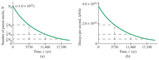
**FIGURE 30–10** (a) The number N of parent nuclei in a given sample of  ${}^{14}_{6}$ C decreases exponentially. We assume a sample that has  $N_0 = 1.00 \times 10^{22}$  nuclei. (b) The number of decays per second also decreases exponentially. The half-life of  ${}^{14}_{6}$ C is 5730 yr, which means that the number of parent nuclei, N, and the rate of decay,  $\Delta N/\Delta t$ , decrease by half every 5730 yr.
