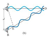
FIGURE 12-17 Sound waves of a single frequency from loudspeakers A and B (see Fig. 12–16) constructively interfere at C and destructively interfere at D. [Shown here are graphical representations, not the actual longitudinal sound waves.]
