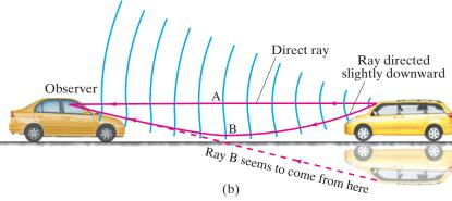
**FIGURE 24–4** (a) A highway mirage. (b) Drawing (greatly exaggerated) showing wave fronts and rays to explain highway mirages. Note how sections of the wave fronts near the ground are farther apart and so are moving faster.
