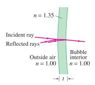
**FIGURE 24–34** Soap bubble, Example 24–11. The incident and reflected rays are assumed to be perpendicular to the bubble's surface. They are shown at a slight angle so we can distinguish them.
