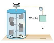
FIGURE 14–1 Joule's experiment on the mechanical equivalent of heat. [The work is transformed into internal energy (Section 14–2).]
