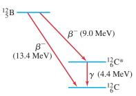
**FIGURE 30–8** Energy-level diagram showing how  ${}^{12}_{5}B$  can decay to the ground state of  ${}^{12}_{6}C$  by  $\beta$  decay (total energy released = 13.4 MeV), or can instead  $\beta$  decay to an excited state of  ${}^{12}_{6}C$  (indicated by \*), which subsequently decays to its ground state by emitting a 4.4-MeV  $\gamma$  ray.
