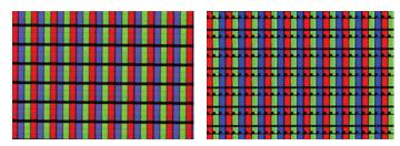
**FIGURE 17–31** Close up of a tiny section of two typical LCD screens. You can even make out wires and transistors in the one on the right.
