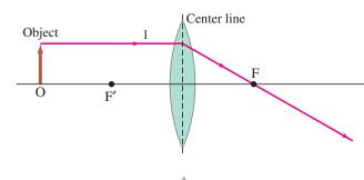
(a) Ray 1 leaves one point on object going parallel to the axis, then refracts through focal point behind
