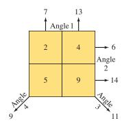
**FIGURE 25–45** A simple  $2 \times 2$ image showing true absorption values (inside the squares) and measured projections.
