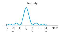
**FIGURE 24–21** Intensity in the diffraction pattern of a single slit as a function of  $\sin \theta$ . Note that the central maximum is not only much higher than the maxima to each side, but it is also twice as wide  $(2\lambda/D)$  wide) as any of the others (each only  $\lambda/D$  wide).
