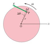
FIGURE 8-4 A point P on a rotating wheel has a linear velocity  $\vec{\mathbf{v}}$  at any moment.
